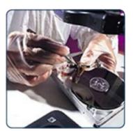
When there is scratching sounds (electric or clicking sounds) or when there has been incidents of physical blows or contamination this indicates the need to directly access the internal components of the hard drive.
